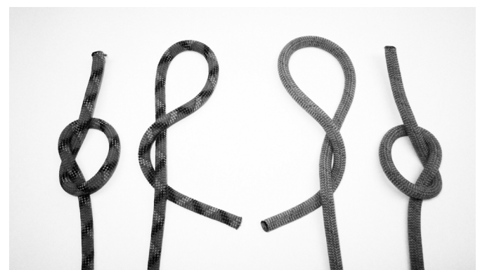
Figure 11. Step 2 – Overhand Knots completed, changing directions to finish Figure Eight Knots with twists or elbows, which look like Crossing Hitches: left S, right Z.
