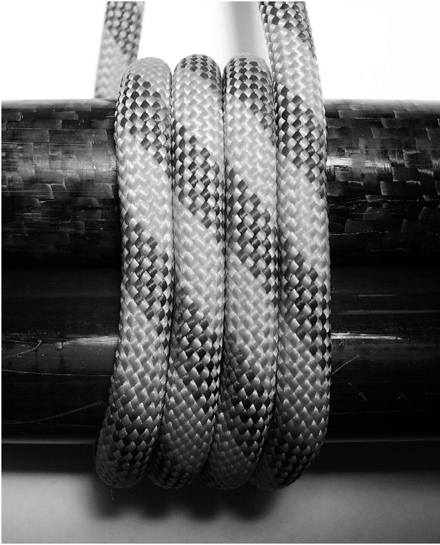
FIGURE 7 Collective Round Turns, which are used to secure limbs together as shown in Figure 4
