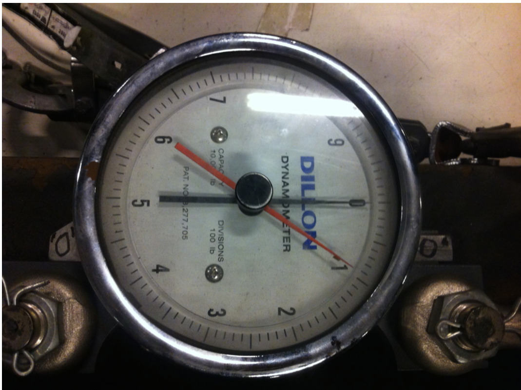
the dynamometer, the red needle shows peak load
