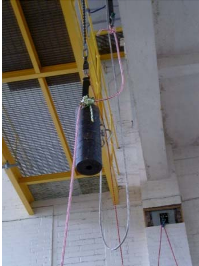
Photograph 12 The single rope drop test rig
