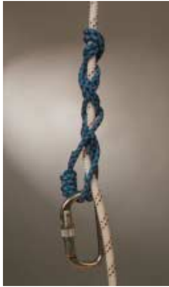
Figure 57 French prusik knot tied with 6 mm accessory cord
