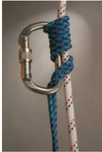
Figure 55 Bachman knot tied with 6 mm accessory cord
