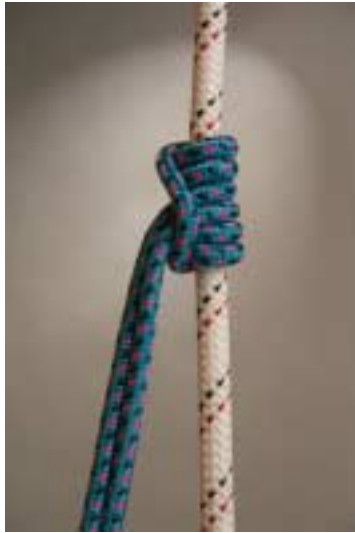
Figure 59 Prusik knot tied with 6 mm accessory cord
