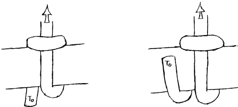
Figure 13: Left: A Münter Hitch with low friction. Right: A Münter Hitch with high friction.
