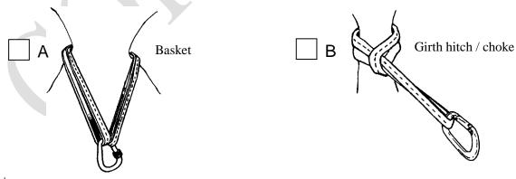
Q14. Study the photos of different types of anchors. Match the descriptor to its corresponding letter. Write letters of the alphabet (A to H) in each of the box's.
