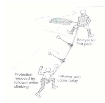
Figure 2.10. Top Rope Belay; fall protection for the second climber
