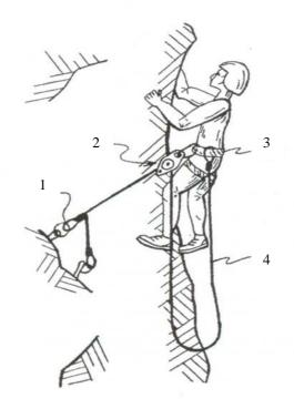
Figure 2.11 Solo Back Roped Rock Climb Showing: Anchor Point (1), Belay Device (2) Harness (3) and Belay Rope (4)
