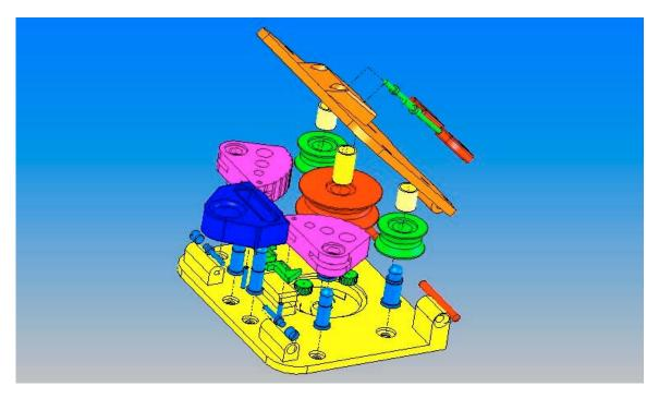
Figure 5.2. SOLIDworks Exploded View of the Back Up Fall Arrest Device Assembly
