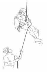
Figure 2.5. Bottom Belay Braking; an abseilers descent can be stopped/controlled by increasing the friction through the descent device by a person pulling on the free ends of the rope.
