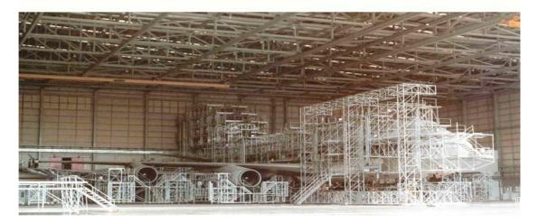
Figure 2.1. Fixed Working Platforms
