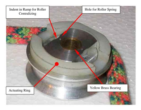
Figure 5.8. Clutch Pulley and Actuating Ring: showing the location of several features for a "trail and error" design evaluation of the operating sizes. A subsequent pulley was made with a smaller roller diameter to provide more effective pulley lock. The redesigned pulley and actuating ring were manufactured to fit the 11mmØ roller size.
