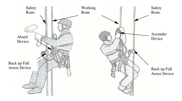
Figure 2.3.(a). Industrial Rope Access Descent. Descender device used on working rope, back-up rope grab used on safety rope. Figure 2.3.(b). Industrial Rope Access Ascent. Ascender devices used on working rope, back-up rope grab used on safety rope.
