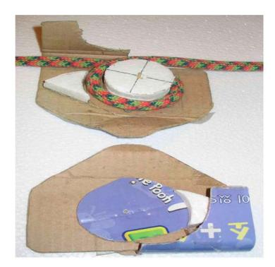
Figure 4.3. Cardboard and Polystyrene Modeling of a Rotating Frame Idea with Integral Blocking Cams on the Inertia Pulley
