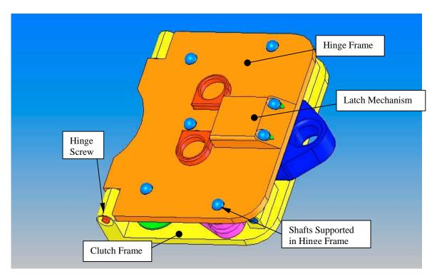
Figure 5.3. Hinge Frame in Closed and Latched Position: showing each shaft that passes through the hinge frame is supported
