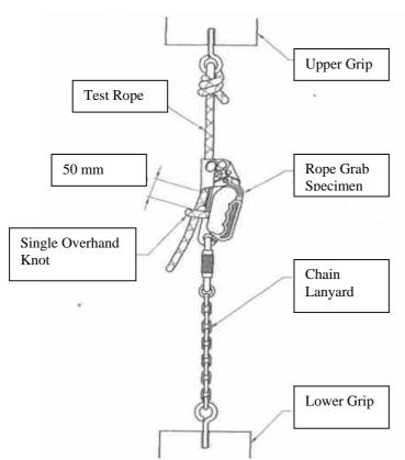
Figure 6.1. Static Test Set Up for Testing Back Up Rope-grab/ Ascender Devices as per Australia/New Zealand StandardAS/NZ4488.1:1997 Appendix A
