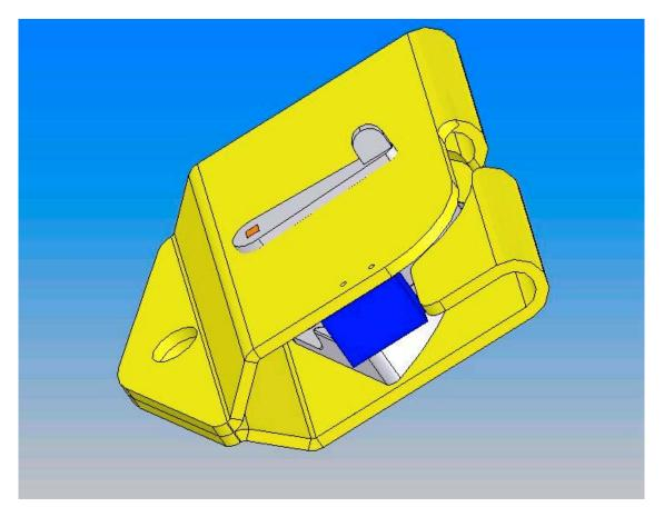
Figure 4.4 The SOLIDworks Virtual Model of the Initial Design Idea. The blue block is a rope guide to prevent the rope from shifting.
