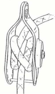
Figure 3.8.(a). Connecting the Safety Rope; a clove hitch is tied in the safety rope.
