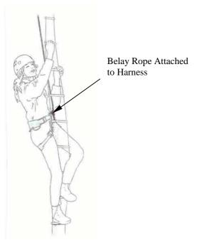
Figure 2.7. Dynamic Rope Belay of a Caver Climbing a Caving Ladder to Provide Fall Arrest.
