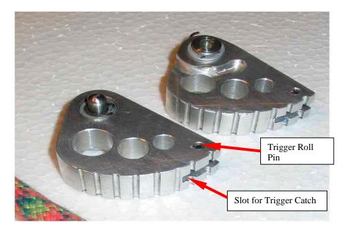
Figure 5.6. The Initial Blocking Cam Units Found to be Too Small
