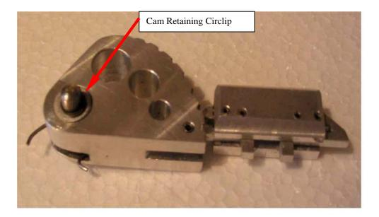
Figure 5.7. The Initial Trigger Release Mechanism: that was resized to accommodate the larger cams. The photograph also shows the blocking cam actuating spring and retaining circlip.
