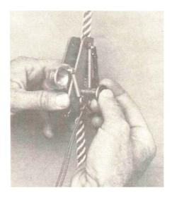
Figure 3.2.(b). Inserting the Quick Release Pin.
