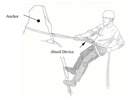
Figure 2.4. Abseiling Descent; a single or double rope is fixed to a solid anchor point, the abseiler is connected by a descender device to the rope and his harness. The abseiler can control his rate of descent by adjusting the friction through the systemby increasing the load with his left-hand grip.
