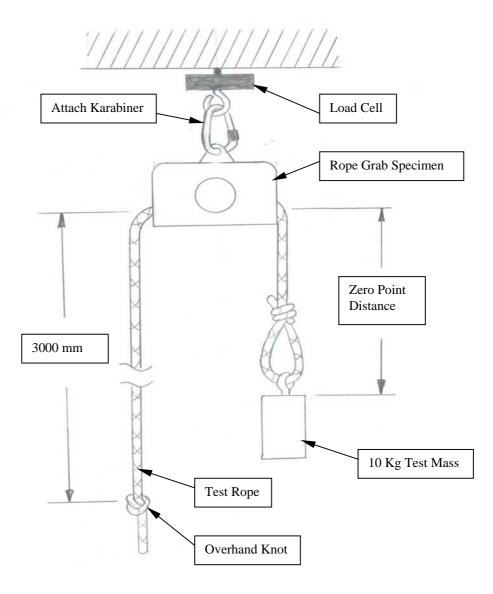
Figure 6.3. Test Set Up for the Back Up Fall Arrest Device Clutch and Cam Release Mechanism Verification Test
