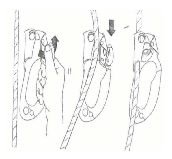
Figure 3.6.(a). Open Cam and Lock Figure 3.6. Stop on Frame Using Thumb
