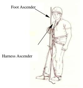
Figure 2.6. Frog Method of Ascender Rope Grab attachment; two ascenders are used – one directly attached to the cavers sit harness, the second to both feet by lanyards/cord. An alternating sit-stand position allows the caver to progressively ascend the rope.
