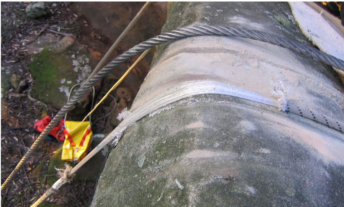
Drop test result - 200kg dropped factor 1/2 fall (3m of rope and 1.5m drop) Sheath parted on the edge. The wire rope in the photo was used to raise the load for the test.
