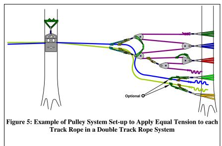
then a maximum of 2 people would pull on this pulley system as per the criteria outlined in #12 above. Note the connector strap between the pulleys connecting the Tandem Prusiks to each track rope. This is used so that the integrity of the pulley system will be maintained, even if one of the track ropes were to fail. Additional anchorage of the track ropes with Tandem Prusiks is
